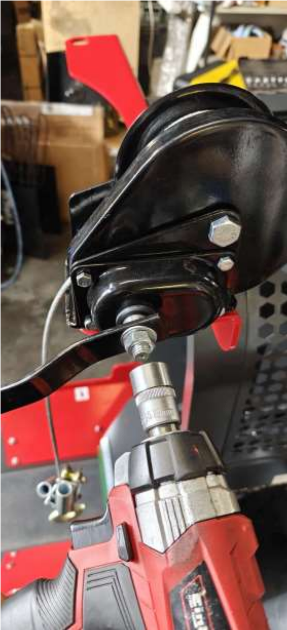
Mounting of winch comb, 19 mm socket.
