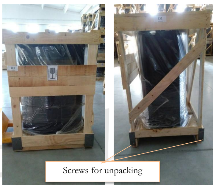
Figure 3 Display of screws to untighten to release the frame
