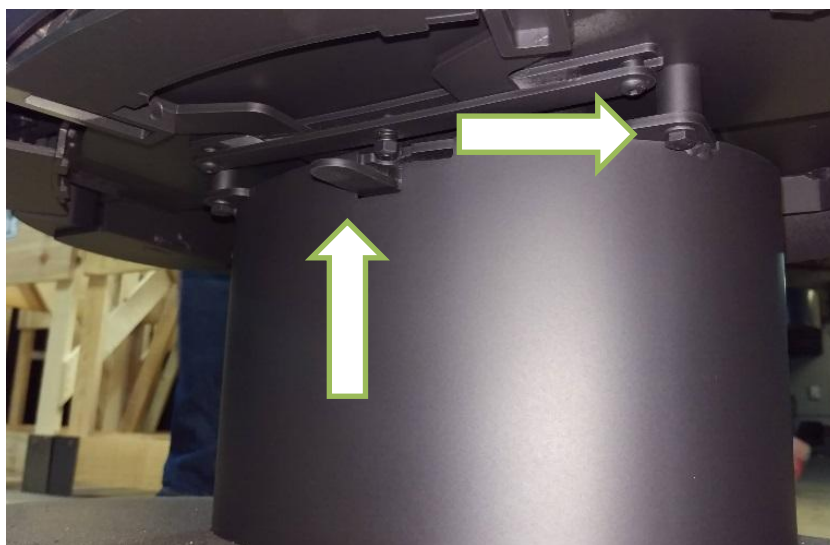
Figure 8 Pedestal stoves' locking lever
