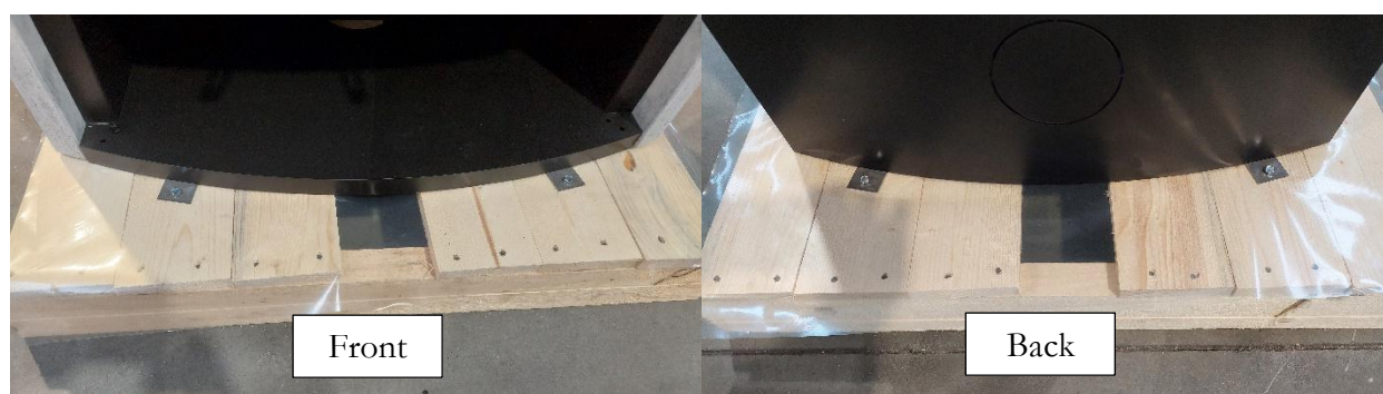
Figure 4 Braces that hold stove to the base which also need to be released.
