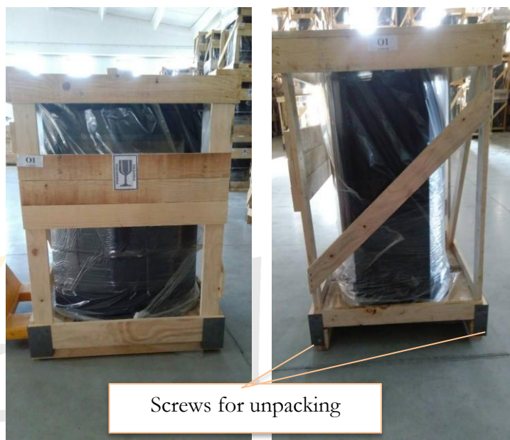
Figure 4 Display of screws to untighten to release the frame
