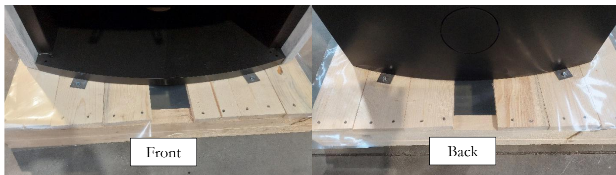
Figure 5 Braces that hold stove to the base which also need to be released.
