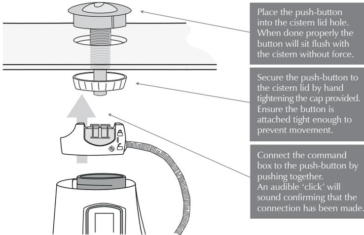
Once the 'command box' has been attached to the push button, lock the device by holding both sides of the coloured tab and pushing upwards until another 'click' sounds.
