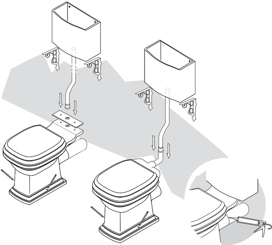
⚠ Operate the flush cycle a few times and continually check carefully for signs of leaks from the inlet valve or toilet outlet if no leaks are evident, your toilet installation is complete.
