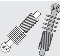
Depending on the water supply pressure, you will need to apply the appropriate restrictor to the threaded tail.
