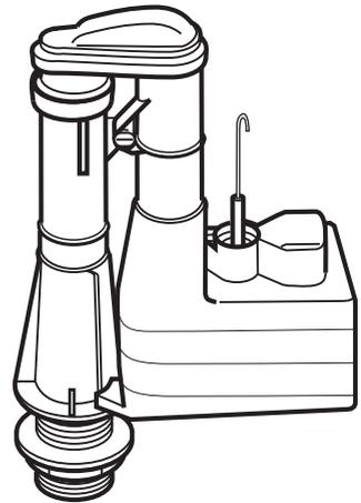
The white downleg connects to the orange bell housing by sliding upwards and securing with yellow linchpin (as pictured.)
