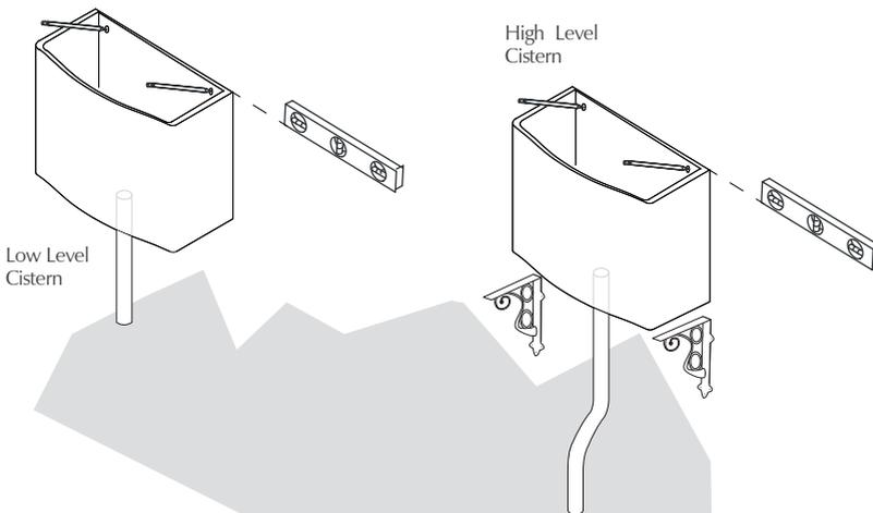
⚠ Once cistern is installed, fit the flush pipe to the bottom of the cistern but do not fully tighten until later in the installation. The flush pipe can be adjusted to fit the space available by removing excess material from either side of the pipe using a saw.
