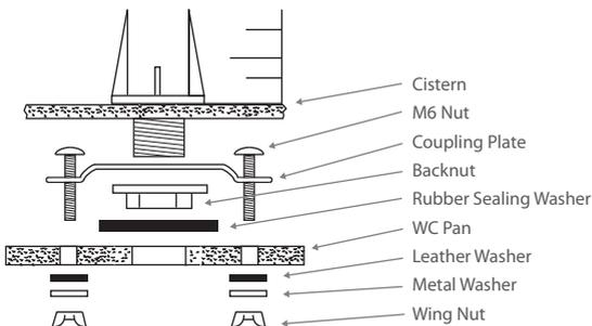
Fit siphon as described earlier but add coupling plate between the cistern and back nut.
