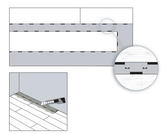
The click elements of the new row, need to be positioned, exactly in the middle of two locks of the previous row. From second row on, always connect the short side first and then the long side.
