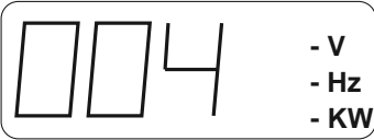
Time (in hours) since generator was first started
