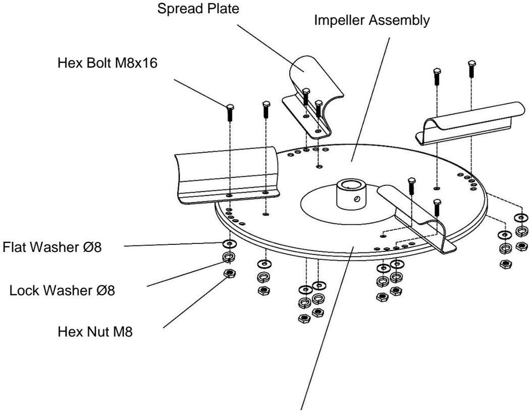
Assemble the Spread Plate to the Impeller accordingly, secure with bolts, washers & nuts.
