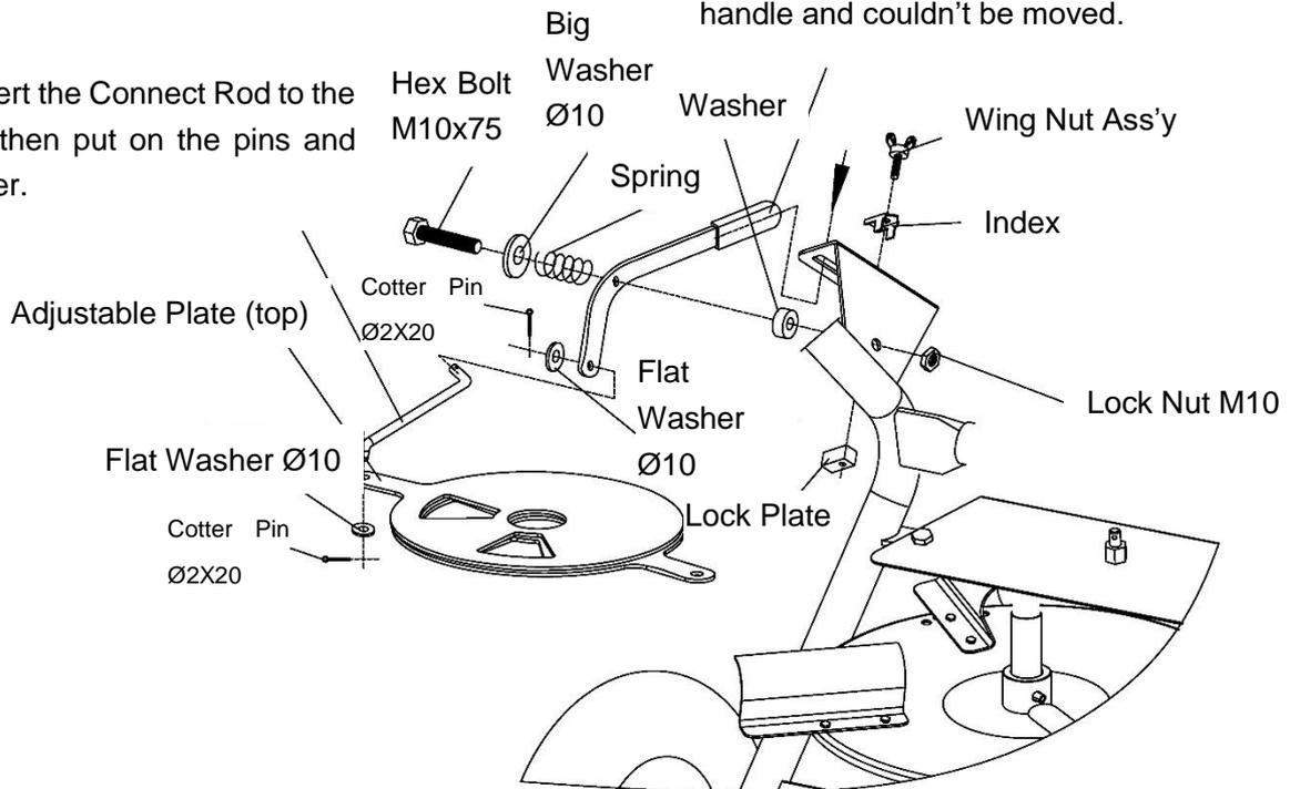
Moving this handle, it could adjust the stuff volume that spreader out on the bottom.
