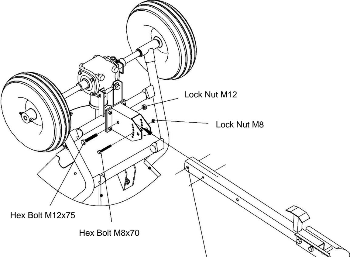
Insert the Hitch Tongue to the Adjustable Plate, let the holes in the same level and then secure with bolts and nuts, tighten.
