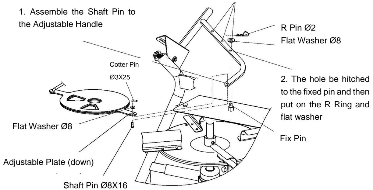
2. The hole be hitched to the fixed pin and then put on the R Ring and flat washer
