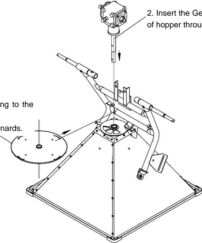
2. Insert the Gear Box into the bottom of hopper through the Impeller.
