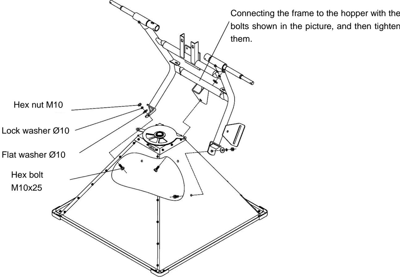
When assembly, please have the hopper side lay, the hopper panel with label should be put in downwards.
