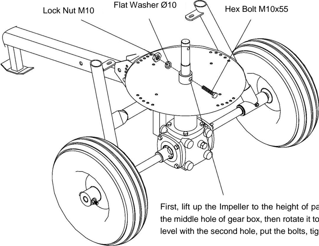
First, lift up the Impeller to the height of parallel with the middle hole of gear box, then rotate it to the same level with the second hole, put the bolts, tighten.
