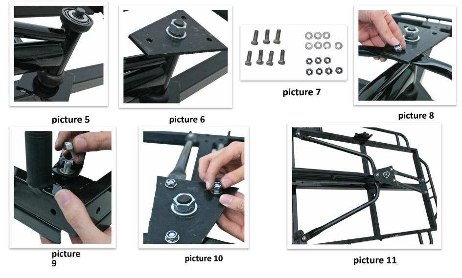
Joint bowlware & bearing & trapezoidal steel plate & washer & spring washer & nut in order and tighten them slightly (see picture 5 & 6); using M8x25 outer hexagonal bolt, washer, nylon nut (picture 7), assemble 2 support steels in order (according to picture 8, 9 & 10) and tighten them firmly (picture 11).
