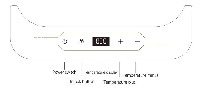
**Power switch:** In the unlocked state, press and hold it for 2 seconds to shut down; when in the locked state, press and hold it for 2 seconds and then turn it on.
