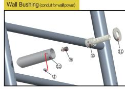
While holding the warmer near the wall, insret the power cord through the Wall Bushing (1) and pull the cord tight from within the wall cavity (see the next pages for ideas on connecting the power cord to power inside the wall)
