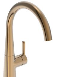
Kitchen faucet with smart dishwasher valve and high swivel spout. Spout's swing angle is factory preset at 120° (can be limited to 0° or 60°). Dishwasher valve closes automatically after 4 or 12 hours (one push opens the valve for 4 hours, pushing for 5 seconds opens the valve for 12 hours). Battery operated, 3 V. There are also in-built limitation options for water temperature and maximum flow-rate. F = with flexible pipes
