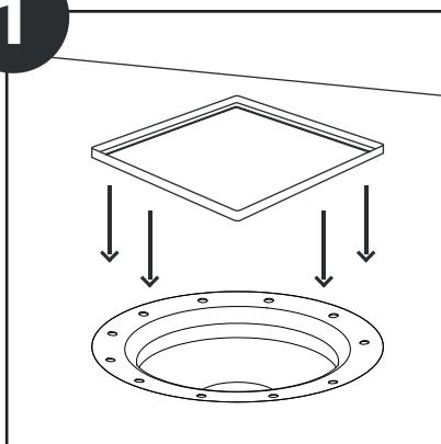
**EN:** The frame is placed centered on the floor drain. Place adhesive under the entire tile frame and push it down onto the floor drain so that the opening coincides with the opening in the floor drain. Make sure that the water trap is free and that the frame is parallel to the surrounding tiles.
