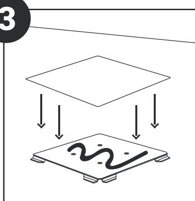
**EN:** The desired tile is attached to the tile holder with wet room silicone or mounting glue for wet rooms. Place the holder in the frame.
